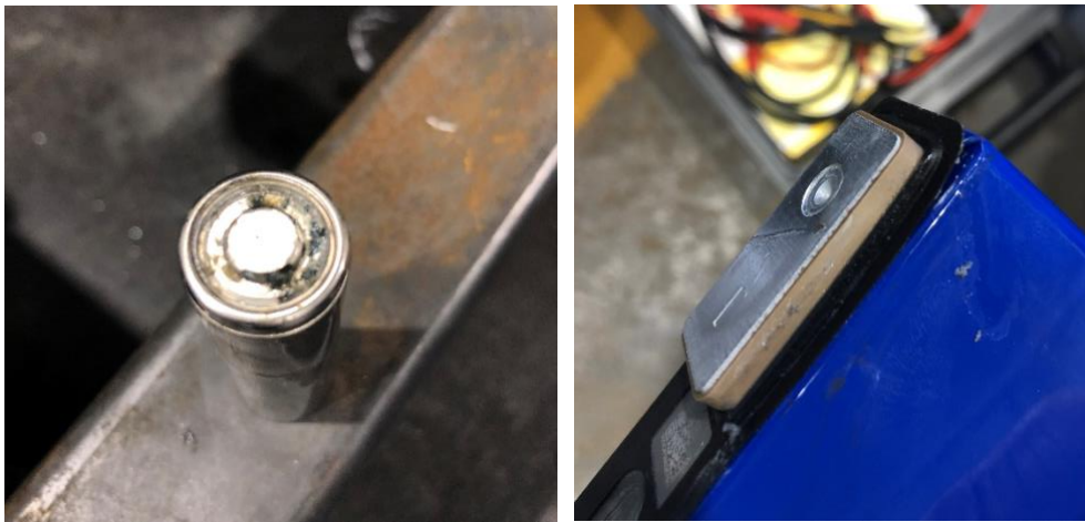
Figure 26. Visible corrosion on the cylindrical cell, but not on the prismatic cell.
