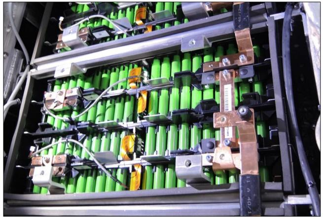
Figure 18: Battery module with battery cells, from the port battery room. Photo: NSIA
