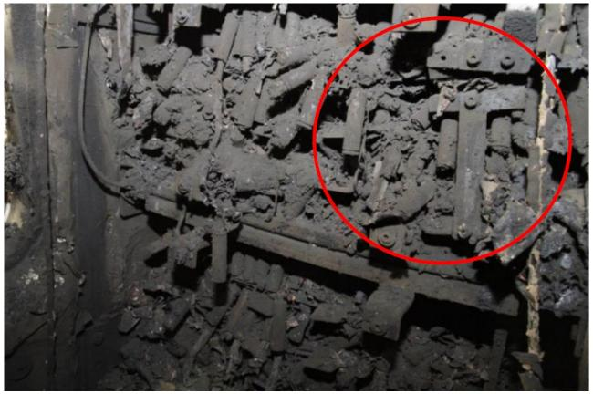
Figure 32: Remnants of battery module 2 in battery stack 6, with the copper strip encircled in red. Photo: Kripos
