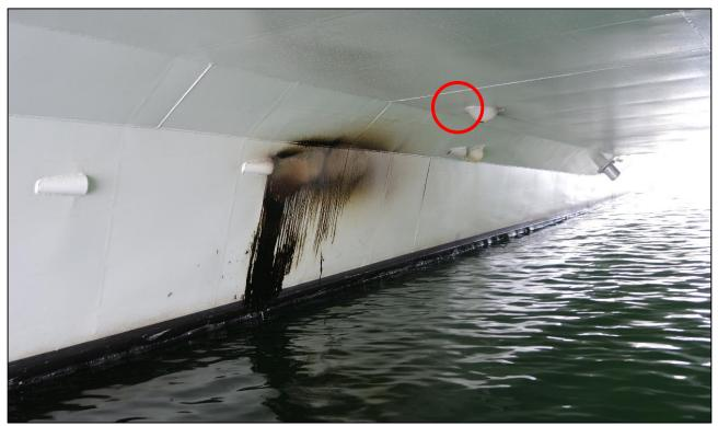
Figure 21: The ventilation outlet from the battery room to the tunnel marked with a red circle. The soot and fire damage inside the tunnel hull came from the cabin at the fore of the battery room. Photo: NSIA
