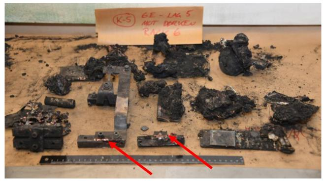
Figure 36: Debris from battery modules 1 and 2 in battery stack 6. The red arrows point to electric arc damage. Photo: Kripos
