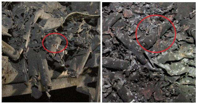
Figure 34: Signs of rupture in the cell wall are encircled in red. Photo: Kripos
