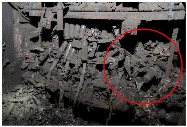
Figure 33: Remnants of battery module 1 in battery stack 6, with the area of the missing copper strip encircled in red. Photo: Kripos
