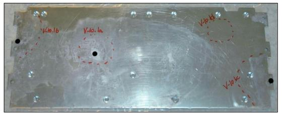
Figure 40: The stack controller's bottom plate. Scraped-off material from the marked areas was sent for analysis. Photo: NSIA
