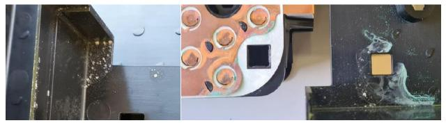
Figure 48: On the left: dried-up crystallised salt inside stack 12, module 5, cell module 2. On the right: visible corrosion and saltwater residue on data bus and cell module cover in stack 12, module 4, cell module 4. Photo: The battery contractor
