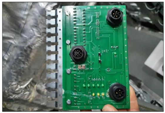
Figure 28: The damaged circuit board that was replaced in stack 12. Photo: The battery contractor
