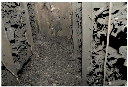
Figure 6: Fire damage to starboard battery room. Photo: Kripos
