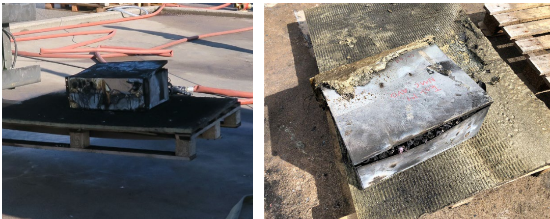
Figure 53 The NMC battery module after Test 10 (left) and Test 14 (right). Note that the module had opened up towards the rear, which is also where the fire was observed to be very intense.
