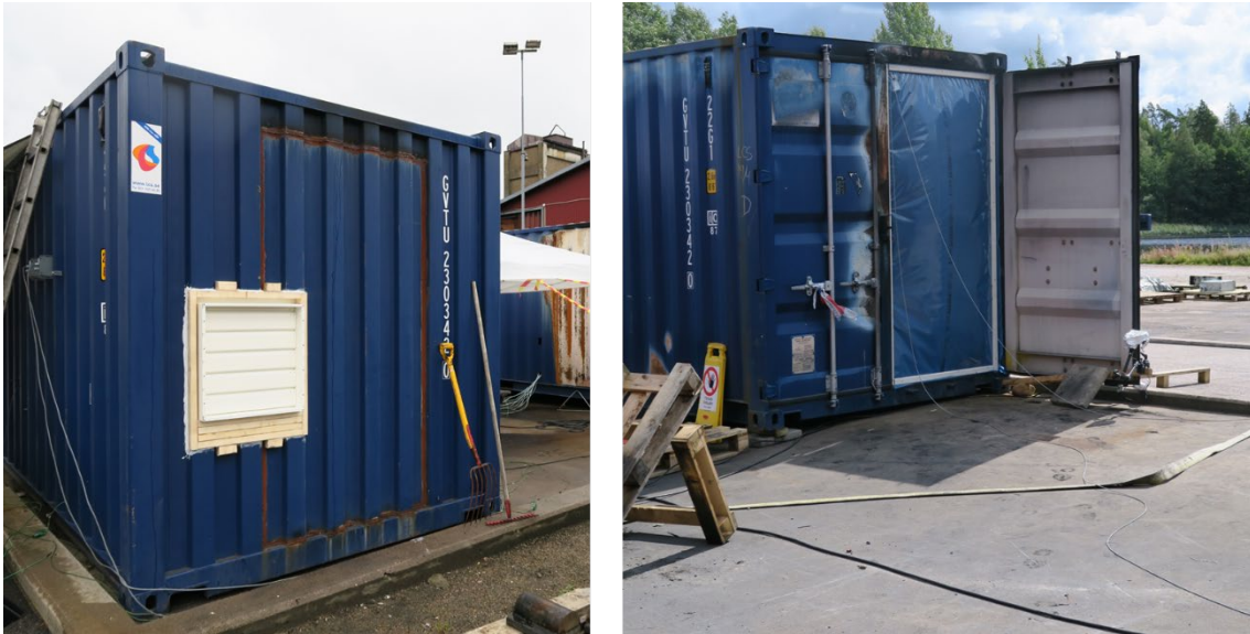
Figure 37 Pressure relief system (left) and plastic sheet used to close-off the container (right)
