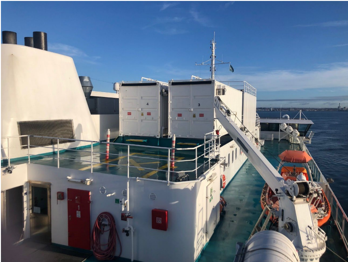
Figure 5 The BESS are located on top of the vessel, inside 32-foot shipping containers.
