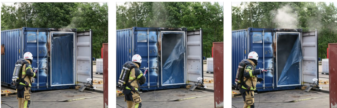
Figure 38 Safely opening the closed container at the end of testing
