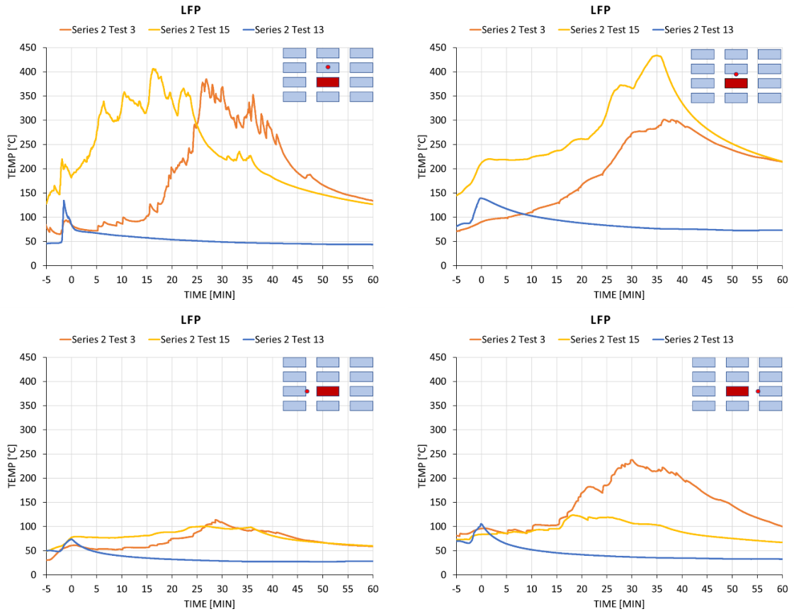
Figure 57. Test results reference test and gas system against LFP module
