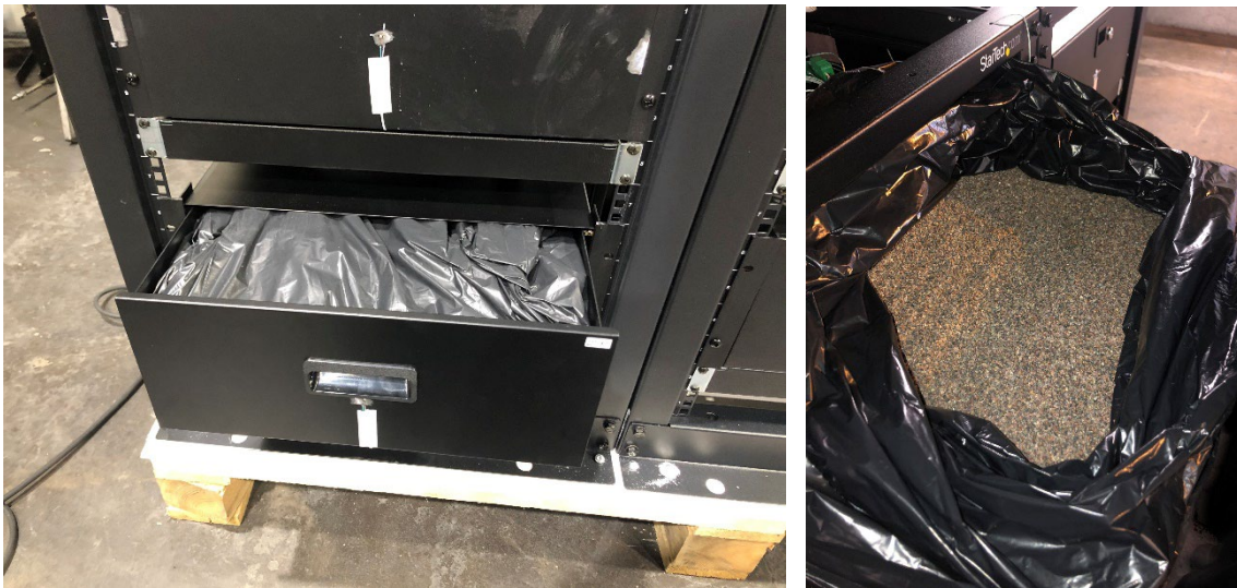
Figure 14 Dummy modules filled with sand
