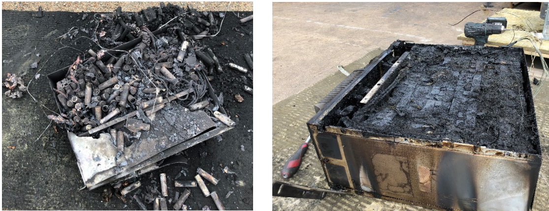
Figure 61 State of the modules after testing, NMC module (left); LFP module (right) after having its lid removed.
