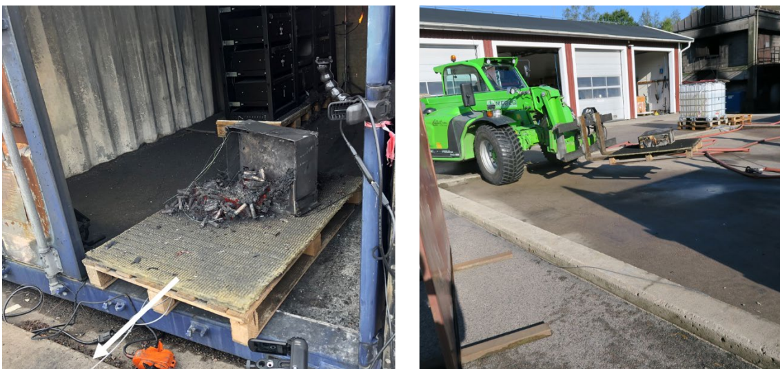
Figure 36 Example of the battery being removed from the container after testing. First the module was pulled onto a pallet, moved to the opening, and then lifted with a machine.
