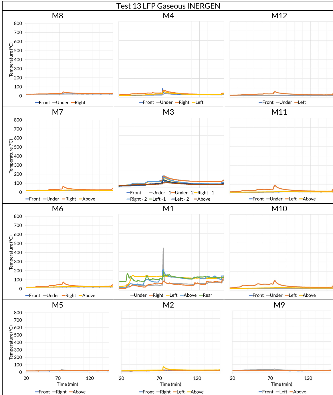
Figure 87 External surface temperatures: Test 13 - LFP -Gaseous INERGEN
